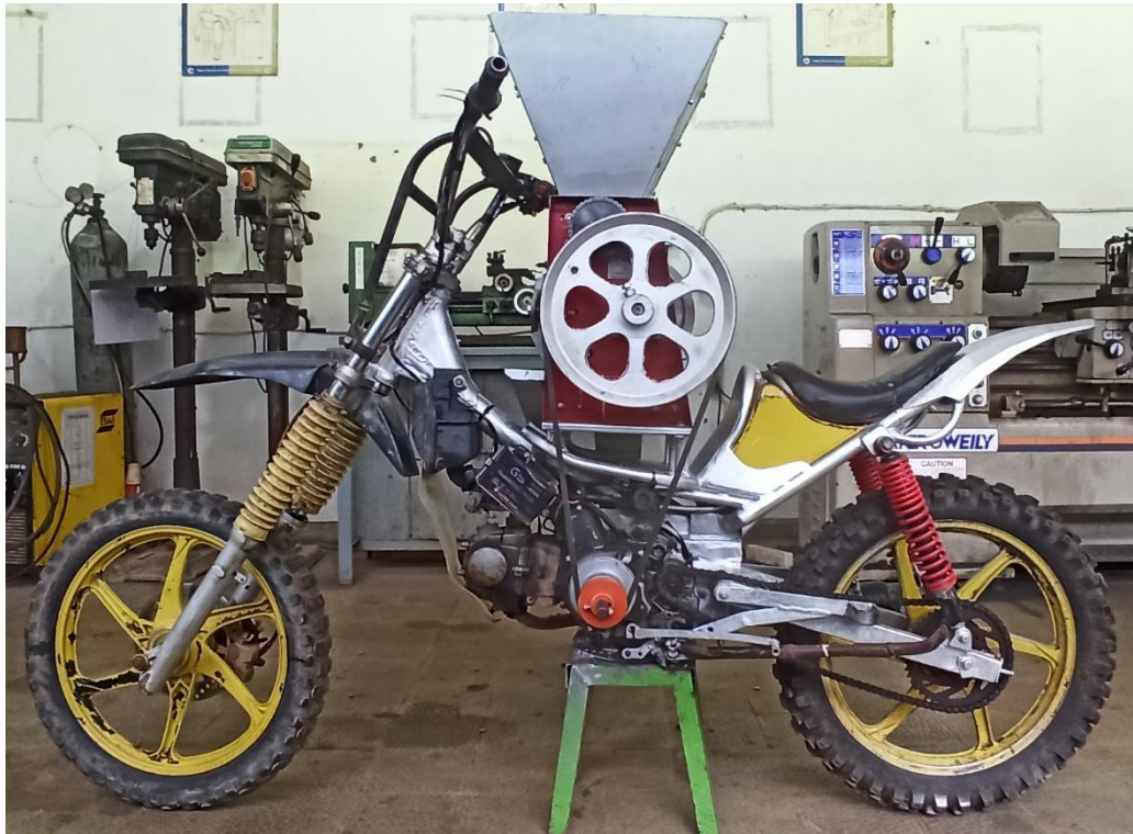
Gambar 55. Mesin pengupas kopi ( pulper ) mobile tampak samping.
