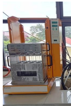
Kjeldatherm Block Digestion Unit
