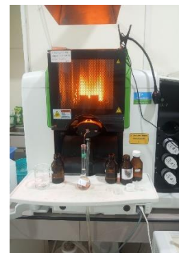
Spektrofotometer Serapan Atom Type PINAACLE900H
