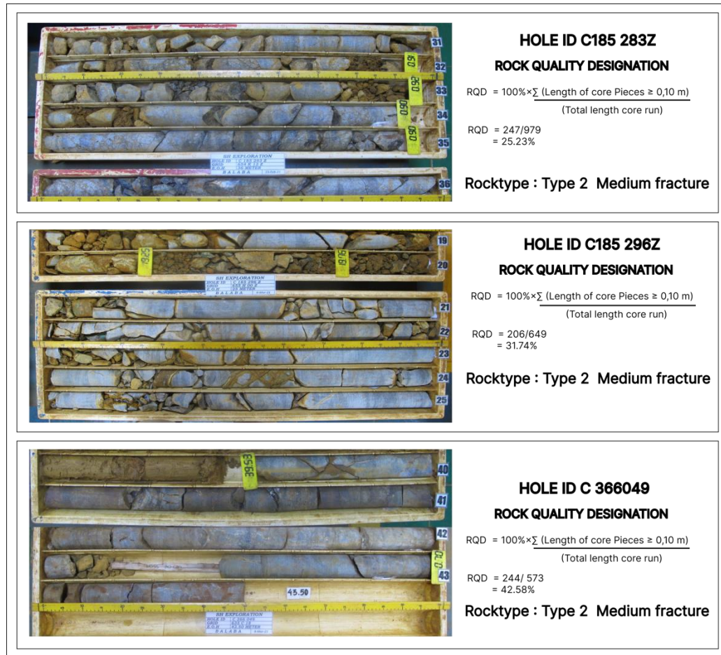
Gambar 4. 5 Batuan dasar Type 2 medium fracture
