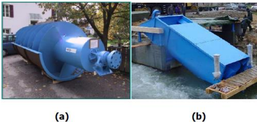
Gambar 1. Tipe Turbin Ulir (a) Tipe steel trough dan (b) Tipe closed Compact Instalation
