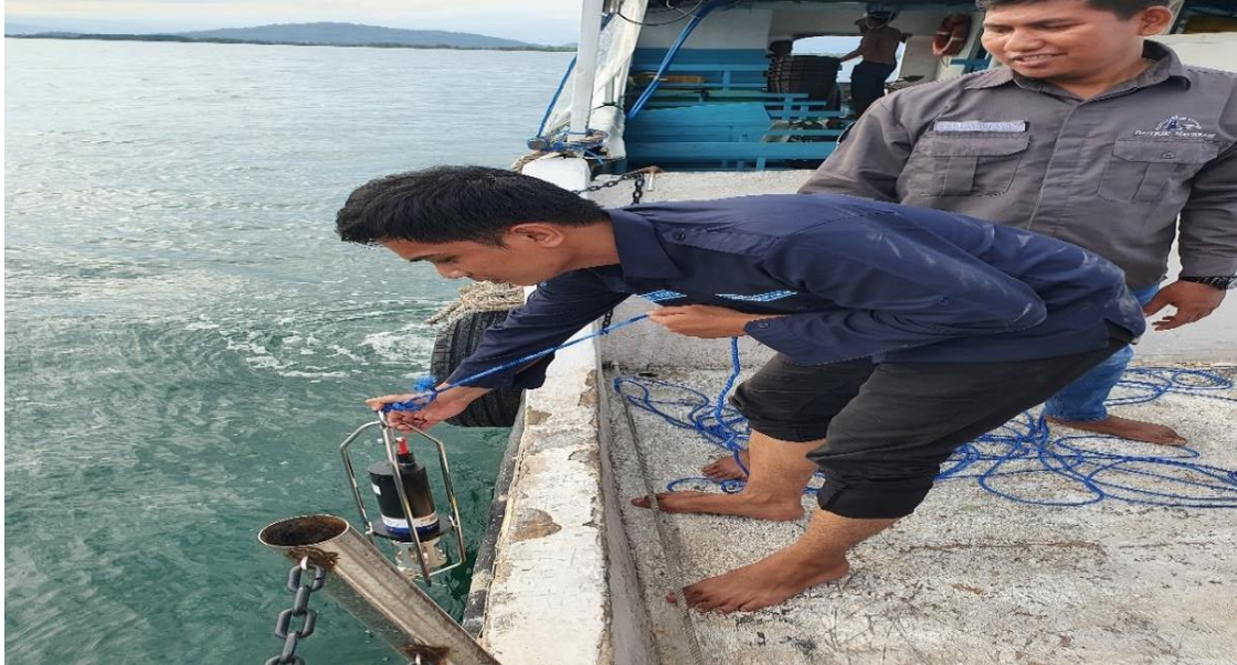
Gambar 4. Proses pengambilan data sound velocity profiler (SVP)
