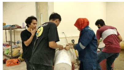
Memasukkan (air + Sikacim Concrete Additive 2% ) kedalam campuran
