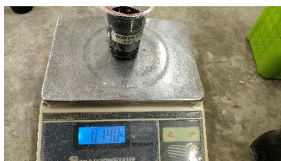
Penimbangan Sikacim Concrete Additive 1,5%
