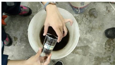
Pencampuran Sikacim Concrete Additive variasi 2% kedalam air
