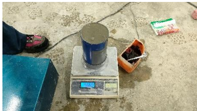
Menimbang berat beton campuran Sikacim Concrete Additive 1,5%
