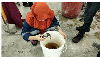
Pencampuran Sikacim Concrete Additive variasi 1,5% kedalam air
