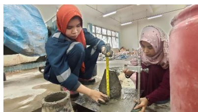
Mengukur tinggi slump campuran Sikacim Concrete Additive 2%
