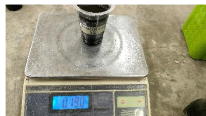
Penimbangan Sikacim Concrete Additive 2%
