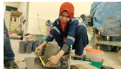
Mengukur tinggi slump campuran Sikacim Concrete Additive 1%
