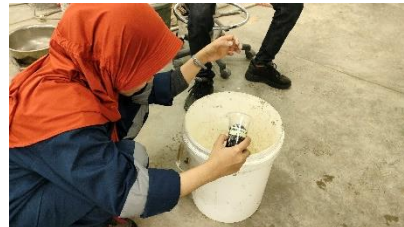
Pencampuran Sikacim Concrete Additive variasi 1% kedalam air
