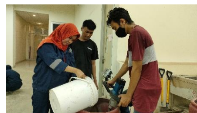
Memasukkan (air + Sikacim Concrete Additive 1,5%) kedalam campuran
