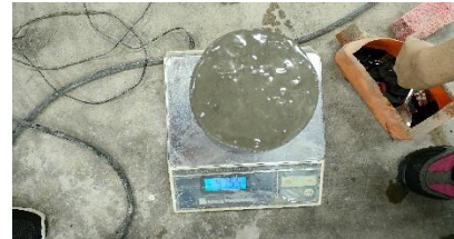
Menimbang berat beton campuran Sikacim Concrete Additive 2%
