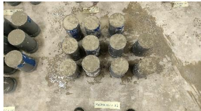
Mendiamkan campuran beton + Sikacim Concrete Additive 2%
