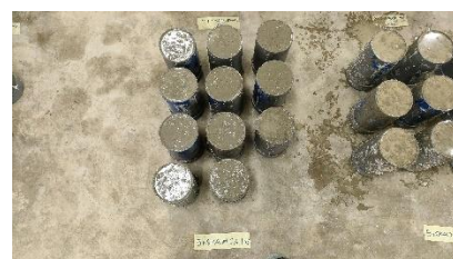
Mendiamkan campuran beton + Sikacim Concrete Additive 1,5%
