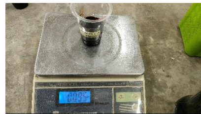
Penimbangan Sikacim Concrete Additive 1%
