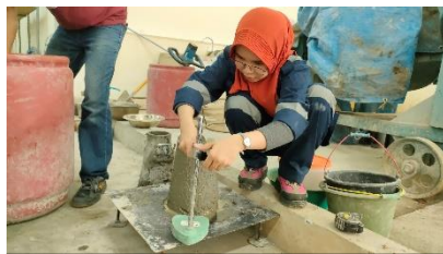
Proses pengujian slump beton normal
