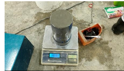
Menimbang berat beton campuran Sikacim Concrete Additive 1%
