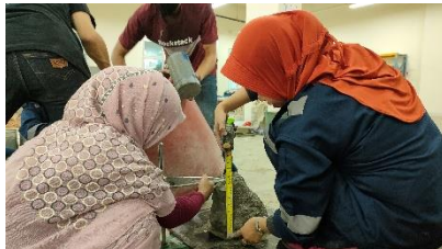
Mengukur tinggi slump campuran Sikacim Concrete Additive 1,5%
