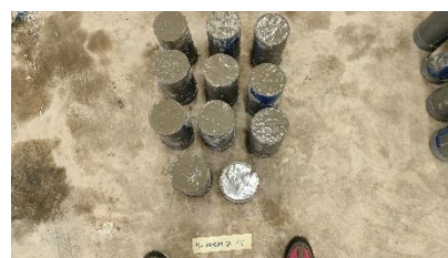
Mendiamkan campuran beton + Sikacim Concrete Additive 1%
