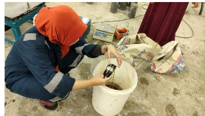
Pencampuran Sikacim Concrete Additive variasi 2% kedalam air
