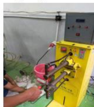
Figure 3. Resistance spot welding machine
