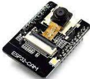
**Gambar 2.4** ESP32-Cam
