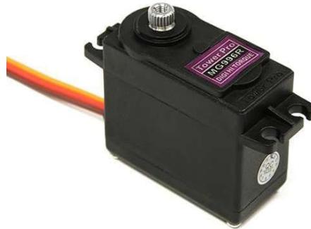
**Gambar 2.6** Servo Motor MG996R (Baihaqi, 2019)
