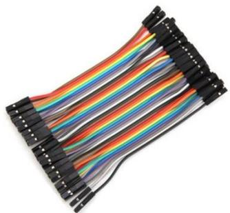
Gambar 12 Kabel jumper *female to female*
