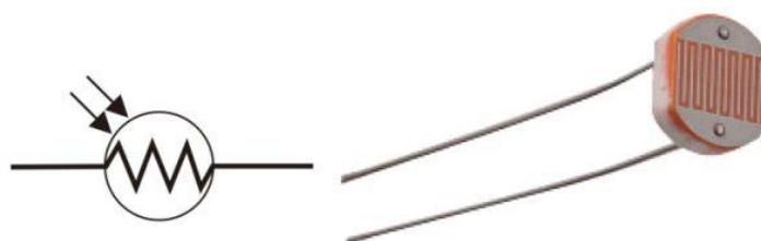
Gambar 4 Sensor light dependent resistor
