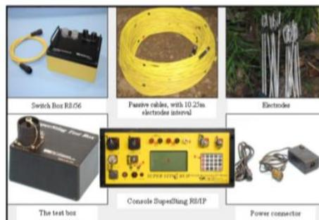
**Gambar 3.2** Kelengkapan instrumen Supersting Multi Channel R8/IP (Artha-Bumi Harapan, 2013)
