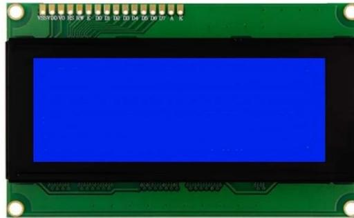
Gambar 8 LCD 20x4
