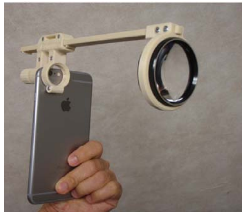
Gambar 30. 3D printed Retinal Imaging Adapter for Smartphones rancangan Dr Hong Sheng Chiong (Hong SC, 2015)
