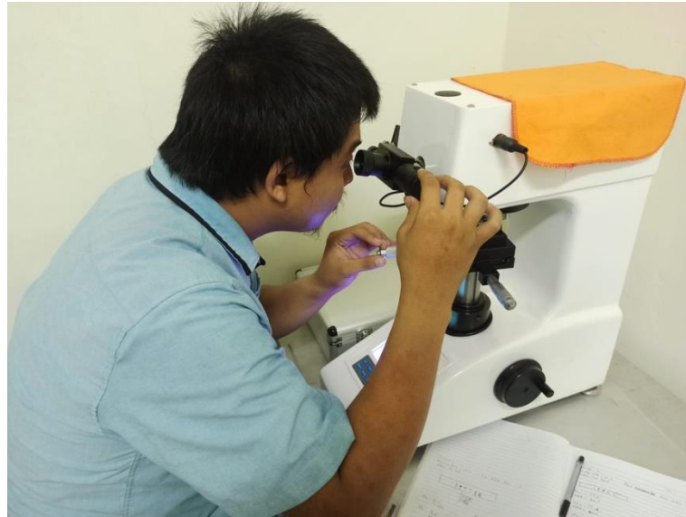
Lampiran 8.1 Pengoperasian alat uji hardness mikro vickers
