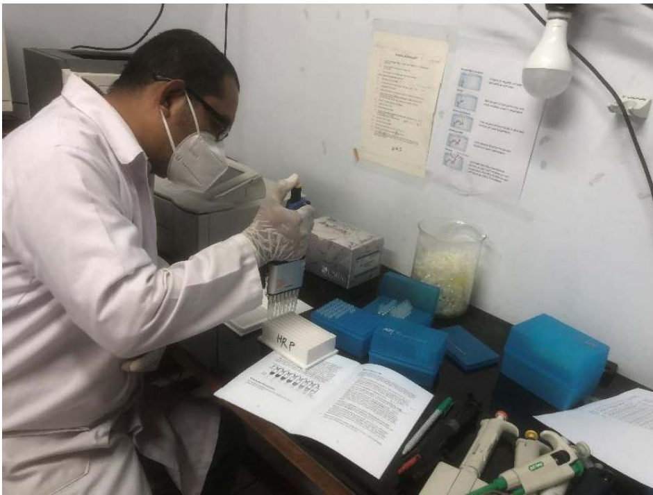
8. Add 100 \mu L Detection Reagen B and Incubate for 30 min at 37 ^{\circ} C
