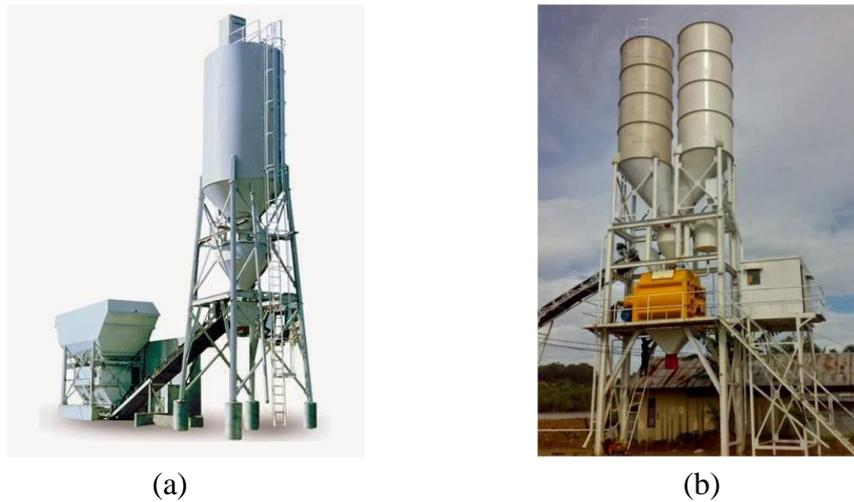
Gambar 6. (a) *Batching Plant Dry Mix* dan (b) *Batching Plant Wet Mix*
