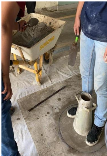
( proses pengujian slump )
