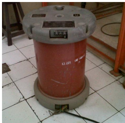
Gambar 3.6 Transformator tegangan tinggi type Tarco Sweden
