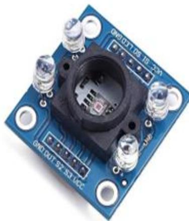
Gambar 7 Sensor Warna TCS3200
