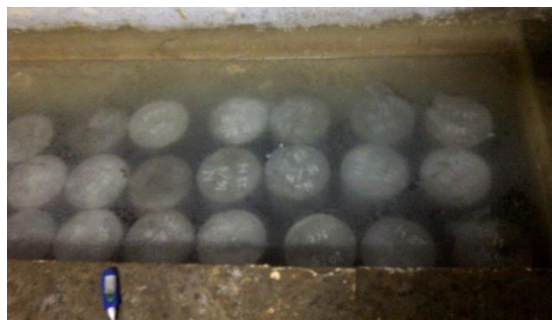
Gambar 3.5 Proses Perawatan ( curing ) Benda Uji
