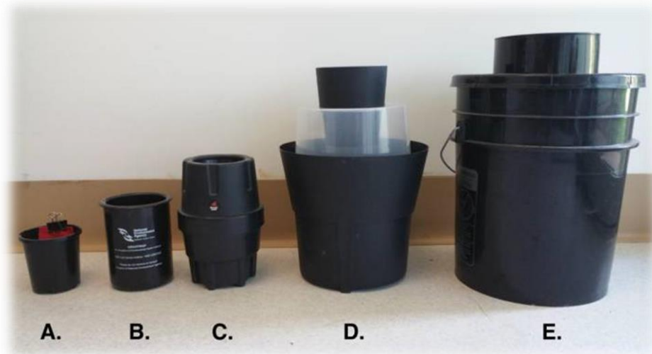
Gambar 2.8 Berbagai bentuk ovitrap (A) Standard (500 mL) lethal ovitrap (LO); (B) National Environmental Agency Singapore sticky ovitrap (SO); (C) MosquiTRAP sticky ovitrap (SO); (D) Biogents Gravid Aedes Trap (GAT); and (E) CDC Autocidal Gravid Ovitrap (AGO). Sumber : (Johnson, Ritchie and Fonseca, 2017).
