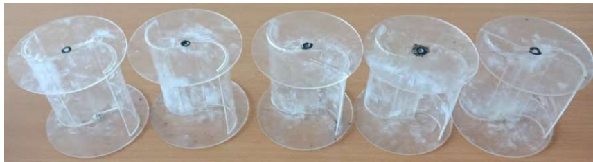
Figure 4. Savonius turbine model for drag coefficient testing.
