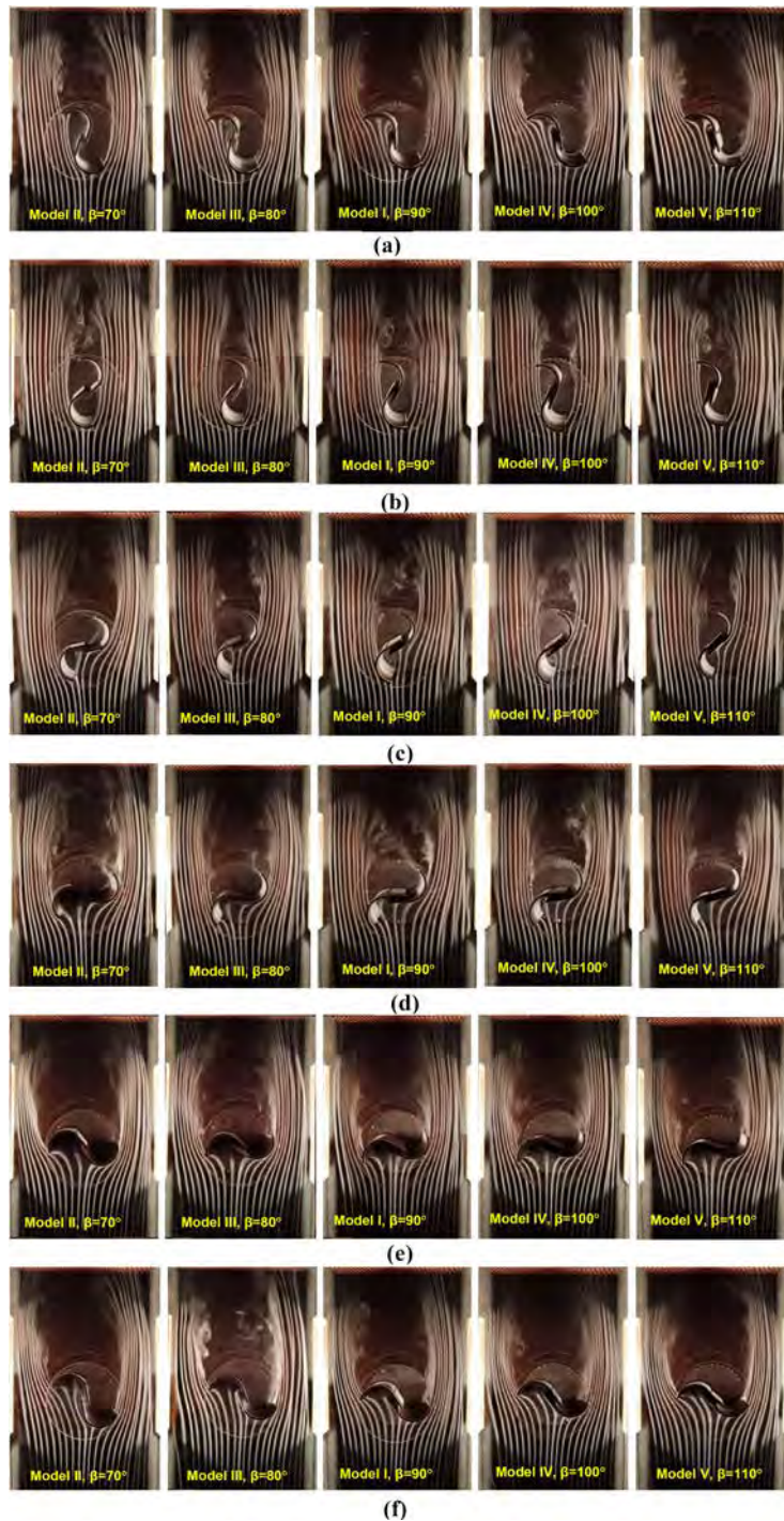
Figure 15. Visualization of flow around the rotor at the rotational angle, \theta : (a) 0^\circ , (b) 30^\circ , (c) 60^\circ , (d) 90^\circ (e) 120^\circ , and (f) 150^\circ .
