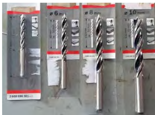
Figure 2. "Brad & spur" drill diameter 4, 6, 8 and 10 mm.
