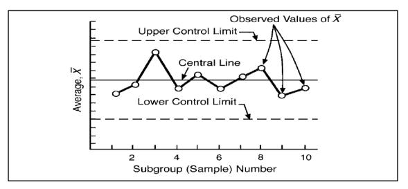
Figure 2.3 Control chart (ASTM International, 2010)
