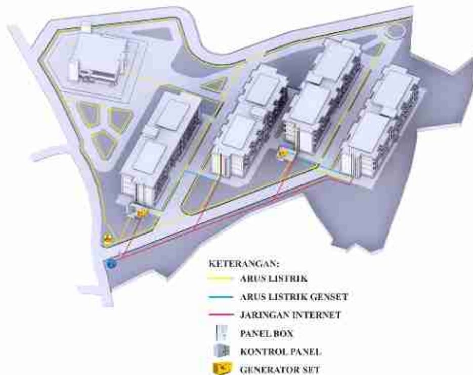
Gambar 11. Rencana Mechanical Electrical
