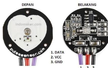
Gambar 2.5 Heart Rate Pulse Sensor
