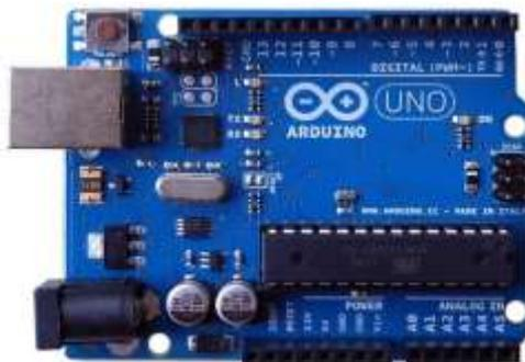
Gambar 2.2. Board Arduino Uno
