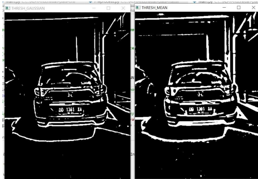
Gambar 3.8 Perbedaan hasil metode threshold . (a) Adaptive Gaussian Thresholding, (b) Adaptive Mean Thresholding.
