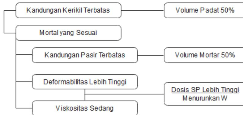
**Gambar 8.** Komposisi campuran *Self-Compacting Concrete*
