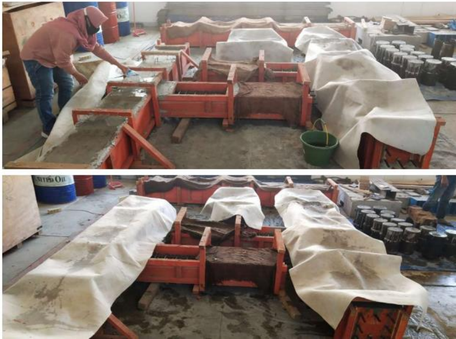
Perawatan Benda Uji (Curing)
