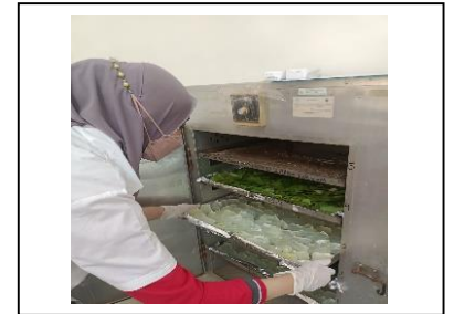
Gambar 6 Proses Pengeringan di Oven Simplisia Temperature 50-60°C
