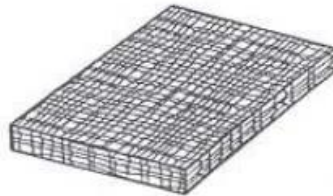
Gambar 2. 3. Woven Fiber composites (Tri Rahmah, 2015)
