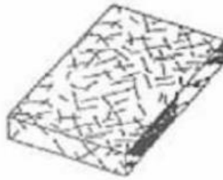
Gambar 2. 4. Discontinuous Fiber composites (Tri Rahmah, 2015)
