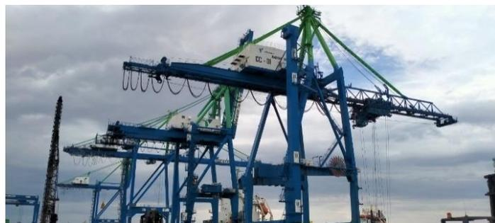
**Gambar 2.14** *Ship to Shore (STS) Crane / Container Crane*
