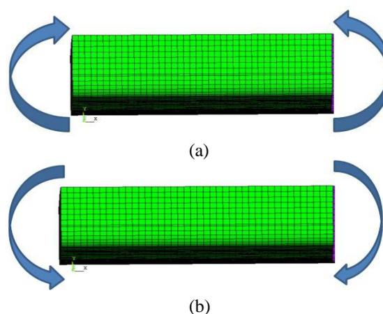
**Figure 3.** Illustration of loading model: (a) sagging condition; (b) hogging condition
