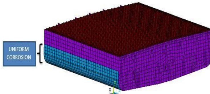
**Figure 2.** FE Model of Ship Hull Compartment
