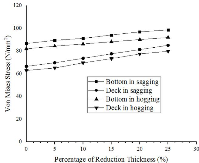
**Figure 6.** Von Mises Stress of All Conditions
