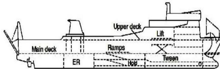
**Figure 1.** General Layout of Ro-Ro Vessel [6]
