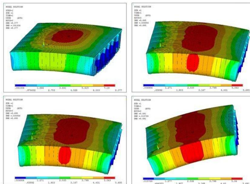
**Figure 4.** Stress Gradations on Hogging Condition
