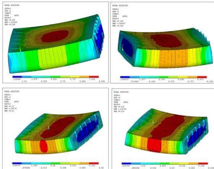
**Figure 5.** Stress Gradations on Sagging Condition
