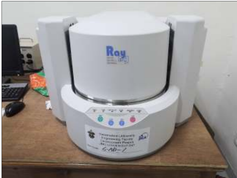
Foto 2.9 Alat analisis X-Ray Flourescence
