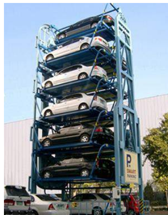
Gambar 2.19 Vertical Rotary Parking System di Jepang Sumber: Intelligent Parking Systems in Japan, 2008
