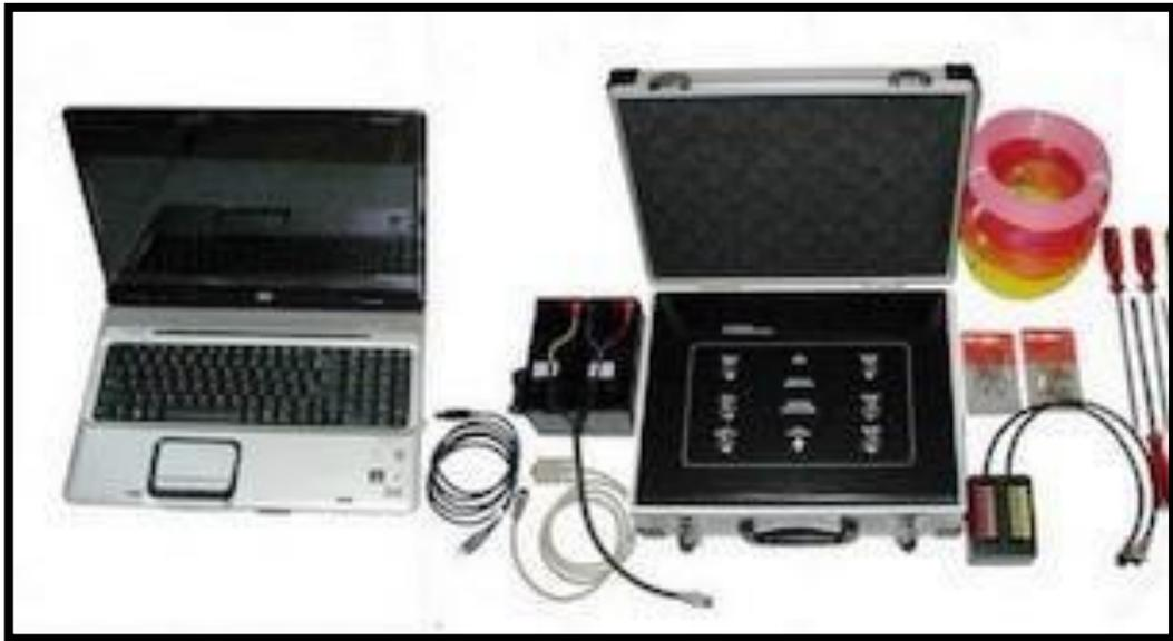
Gambar 1.2 Resistivitymeter S-Field Multichannel dan laptop
