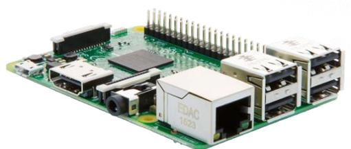
*Gambar 2.8 Gambar Raspberry Pi 3 B+*
