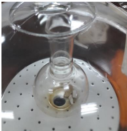
Proses pengukurab bobot tetap (Analisis kadar lemak metode soxlet )
