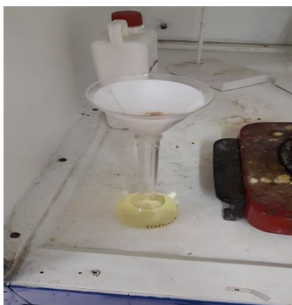
Proses pengukurab bobot tetap (Analisis kadar lemak metode soxlet )
