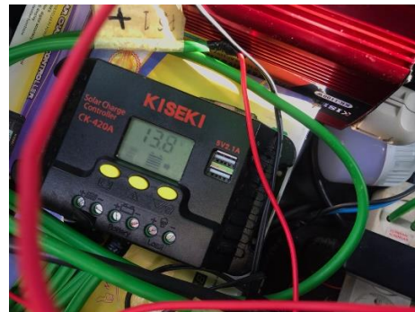
Solar Charge Controller
