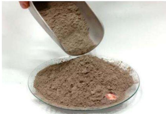
**Gambar 1.** Abu terbang kelas F
