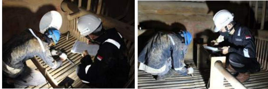
A.2 Gambar pengukuran dimensi economizer tube , (A) economizer tubes baris ke 7 dan (B) economizer tubes baris ke 10.
