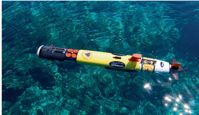
Gambar 2. REMUS 100 AUV di Glovers Reef, Belize [9].
