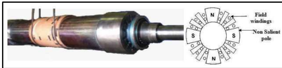
Gambar 2.13 Non Silent Pole Rotor (Yuniarti & Prianto, 2010)
