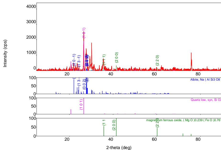
Lampiran 22. Hasil analisa XRD mortar B (10% trass) umur 28 hari
