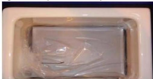
**11.8:** The polystyrene lid is placed on top of the box. The lid of the plastic outer box is closed. Every Tuesday a datalogger is placed in both the large transport box and the Mediporter ([Section 13](#)).
