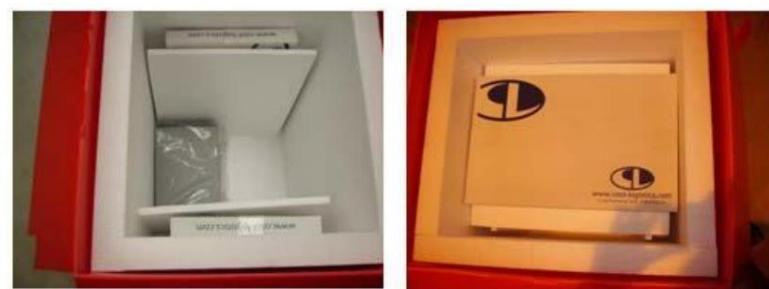
**11.7:** A third spacer is placed on top once the sample racks are all loaded and the
