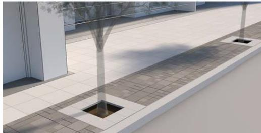
**Gambar 20.** Parit Tertutup (*Covered Soil Trench*)
