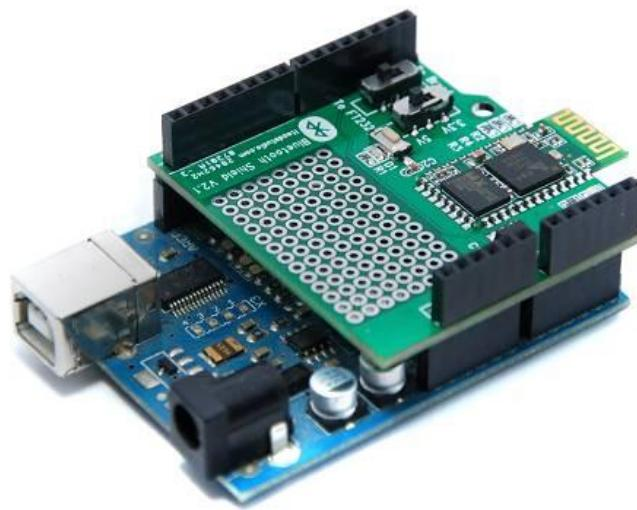
BT Shield V2.1 is a Serial port Bluetooth module (Slave) breakout board, and it's compatible with Arduino and IFlat-32, it can directly plug in with Arduino/IFlat-32 board, use the UART port for communicating to Arduino/IFlat-32 or FT232.
