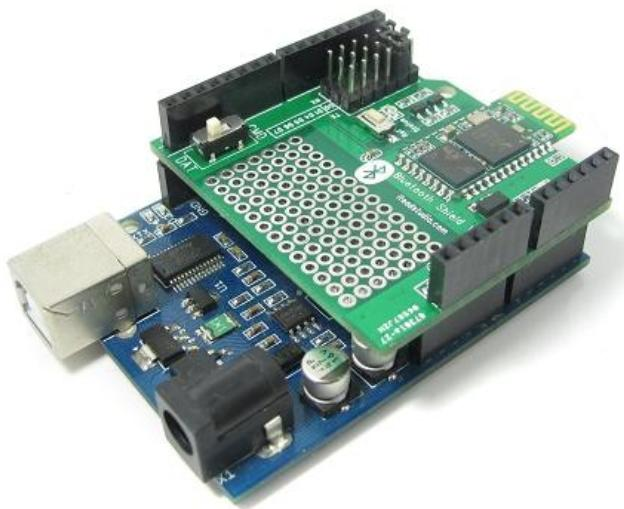
BT shield V2.2 is a serial port Bluetooth module (with master and slave mode) breakout board, it's compatible with Arduino and IFlat-32, it can directly plug on Arduino/IFlat-32 board, use UART port for communication with Arduino/IFlat-32 or PC.
