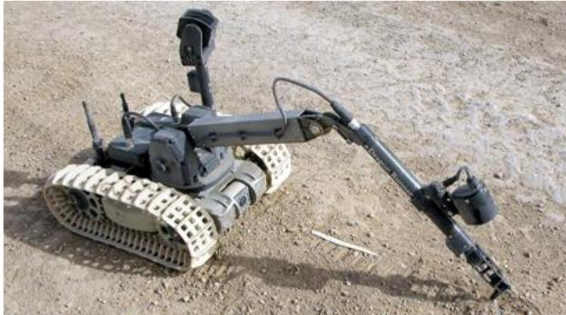
Gambar 3. Robot Mobile Manipulator beroda caterpillar
