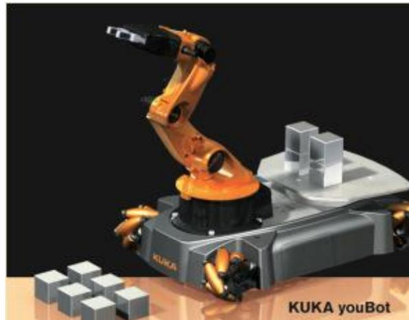
Gambar 4. Robot Mobile Manipulator Beroda Omni
