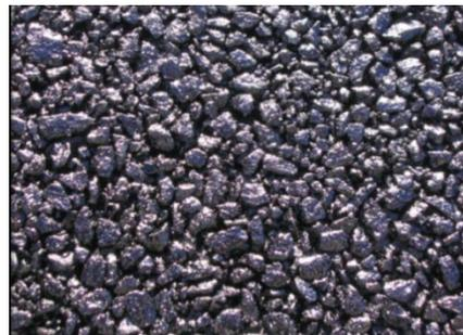
**Gambar 2.5** Permukaan Aspal Porous (\*UNHSC Design Specifications for Porous Asphalt Pavement and Infiltration Beds)
