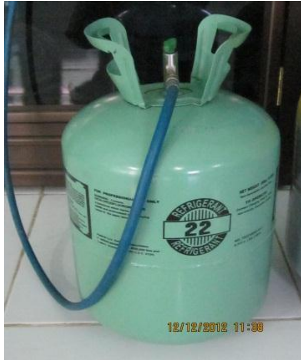
Gambar A.1 Refrigeran R22
